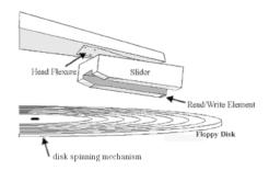
The head is always positioned above one of the 40 tracks. The head can slide radially: *forward* (toward the center of the disk) or *backward* (toward the edge of the disk).
